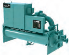
YMC² Water to water heat pump Variable speed centrif. compr. / R134a Magnetic bearings / R134a Hot water up to 65°C Heating cap.: 1600 to 2800 kW
