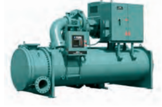
YK HP Water to water heat pump Centrifugal compr. / R134a Hot water up to 50°C (Std) & 70°C (HP) Heating cap.: 1000 to 9000 kW
