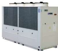
YLHA Air to water heat pump Scroll compressor / R410A Hot water up to 50°C Heating capacity: 12 to 150 kW
